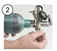
Tighten the tee screw on the regulator by turning the handle clockwise.
