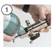
Slide the regulator over the neck of the cylinder, and line up the pins on the regulator with the holes in the cylinder neck.
