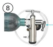
Open the cylinder air flow valve.
