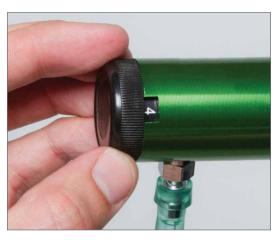
**5** Rotate the barbed outlet flow regulator to 4 LPM.
