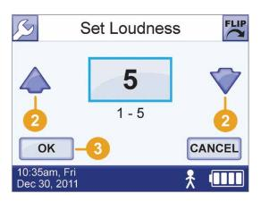
2 Touch the **Up** arrow to increase the volume level or the **Down** arrow to decrease it. If you press and hold an arrow, the number automatically increases or decreases.
