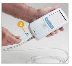
**2** Plug the interface into the ventilator port.
