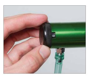
**3** Ensure the barbed outlet airflow gauge is set to 0.
