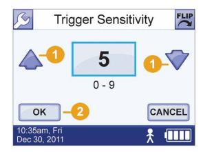
1 On the **Trigger Sensitivity** screen, touch the **Up** arrow to increase the value or the **Down** arrow to decrease it. If you press and hold an arrow, the number automatically increases or decreases.
