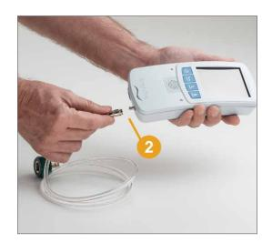
**2** Push the small oxygen supply hose connector onto the oxygen supply connection until it snaps into place.
