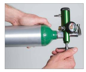
**2** Tighten the tee screw on the regulator by turning the handle clockwise.
