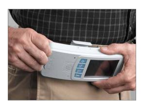
**2** Line up the belt clip with the ventilator sockets, and push down until the clip audibly snaps into place.
