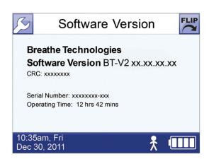
The screen displays software version, serial number, and total operating time.
