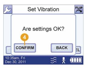
4 In the message asking if the settings are **OK**, touch **Confirm**, and check that the **Vibrate** icon **⋦** appears at the bottom of the touch screen, indicating the ventilator is in vibrate mode.
