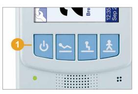
1 Turn the ventilator off by firmly pressing the **Power** button for about three seconds.
