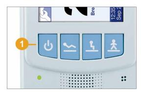
**1** Press the **Power** button to turn on the ventilator.
